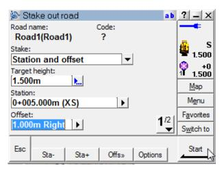
Select the chainage and offset you want to setout and you should have a displayed a bearing and distance to that point as shown below.
